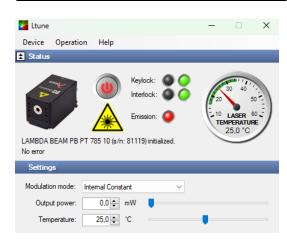
All operating parameters can be monitored and controlled from a PC using the Ltune laser control software for Windows. Alternatively, the laser can easily be controlled from your own application software. Please refer to the user manual for a detailed description of the communication protocol. You can find downloads on our website
