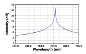
This is a typical emission spectrum of a VHG-stabilized 785nm 50mW pigtail Laser
