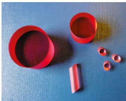
$\text{Al}_2\text{O}_3:\text{Ti}^{3+}$  – titanium-doped sapphire crystals combine outstanding physical and optical properties with broadest lasing range.
