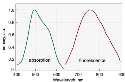
The absorption band of Ti:Sapphire centered at 490 nm makes it suitable for variety of laser pump sources – argon ion, frequency doubled Nd:YAG and YLF, copper vapour lasers. Because of 3.2  $\mu\text{s}$  fluorescence lifetime Ti:Sapphire crystals can be effectively pumped by short pulse flashlamps in powerful laser systems.
