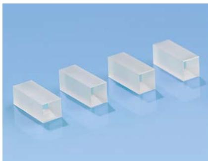
Nd:KGW crystals are low lasing threshold, highly efficient laser material exceptionally suitable for laser rangefinding applications. The efficiency of Nd:KGW lasers is 3–5 times higher than the one of Nd:YAG lasers. Nd:KGW laser medium is one of the best choices ensuring effective laser generation at low pump energies (0.5 – 1 J). These crystals supplied by EKSMA OPTICS feature high optical quality and great value of bulk resistans for laser radiation.
