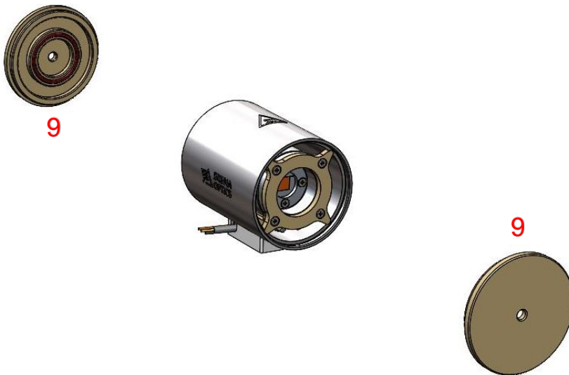
Figure 8. HP200 oven assembly step 4
