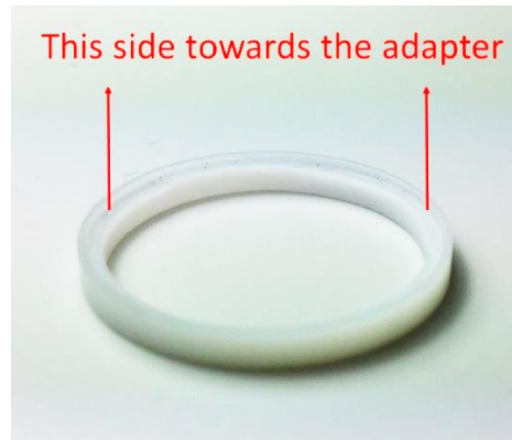
Figure 4. Orientation of Teflon gasket
